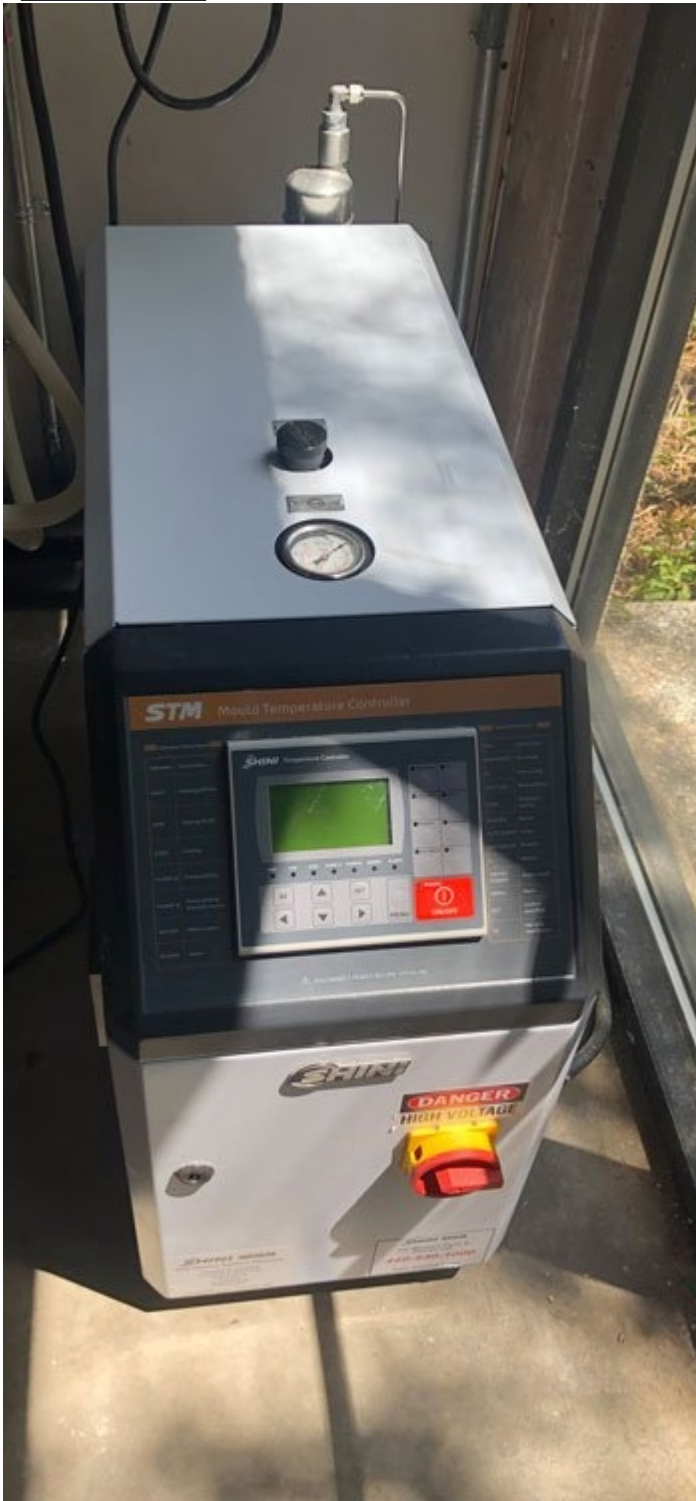
This is a front view look at the hot mineral oil heater. Note that it is placed very close to the wall.
