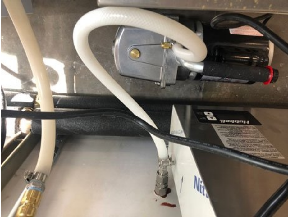
A top view of the vacuum pump with braided silicone hose going to a hose barb on the wall.
